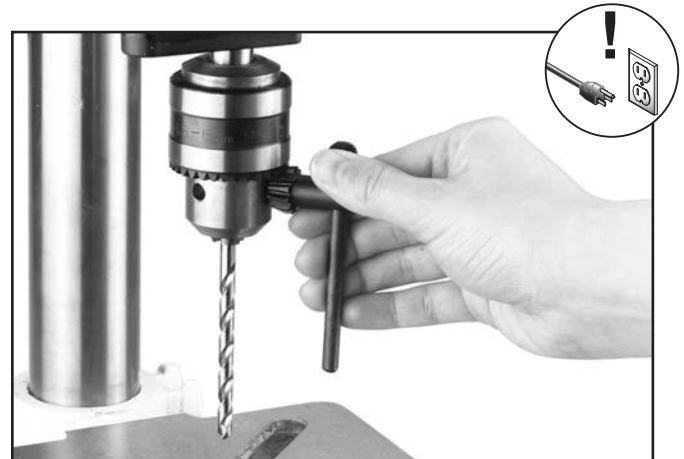
Figure 36. Example of tightening chuck.
