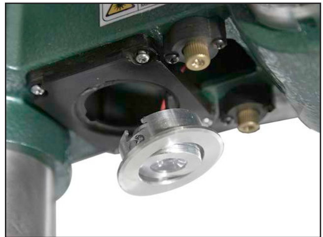
Figure 90. Laser module and LED wiring.
