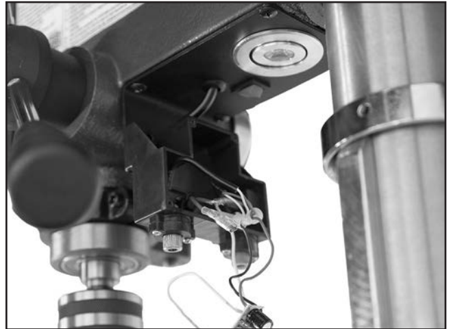
Figure 86. Laser module electrical box attached to LED assembly.
