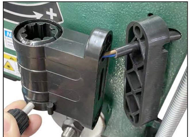
Figure 91. Chip guard micro switch wiring.
