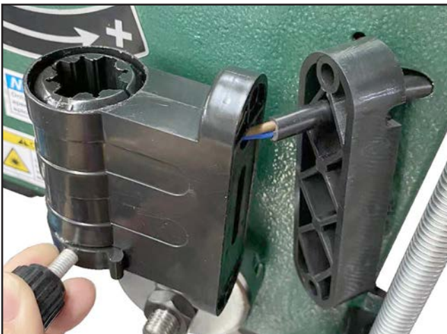
Figure 94. Chip guard micro switch wiring.
