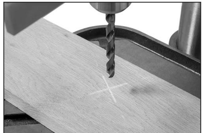
Figure 48. Example of laser crosshairs aligned with indentation on workpiece.
