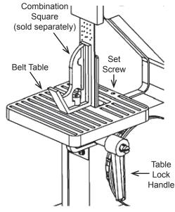
Figure G: Adjusting the Belt Table
