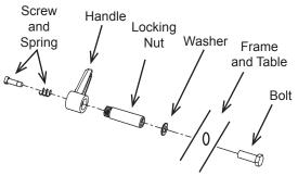
Figure F: Installing Handle
