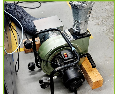
Exhaust Blower and Filter Box
